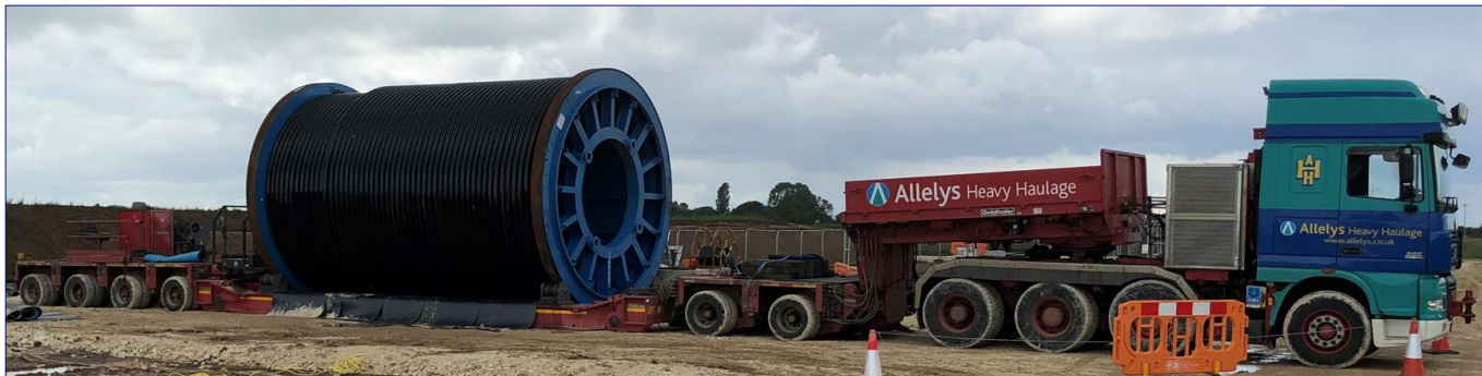
Figure 4.3: Example Cable Delivery AIL
