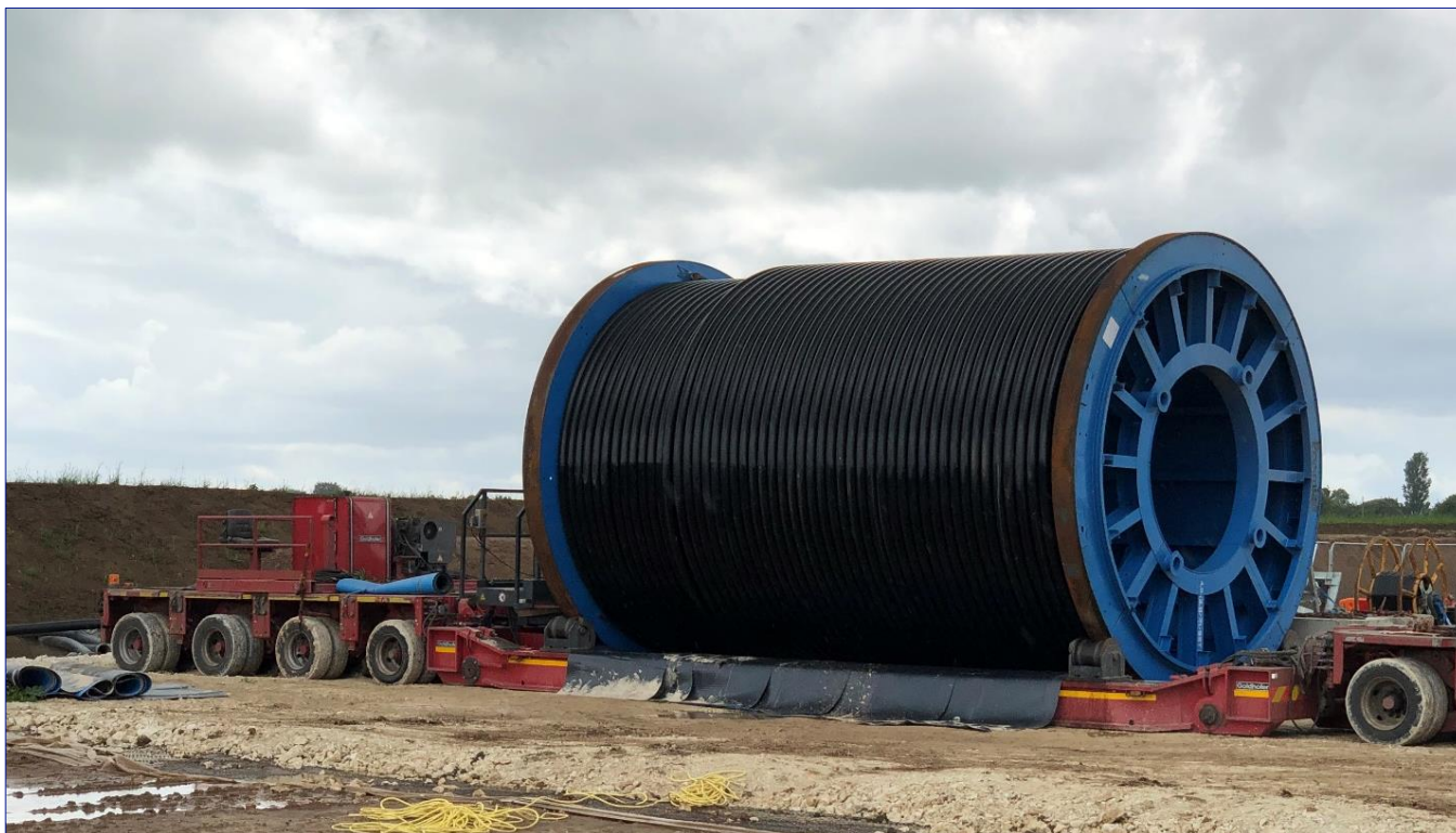
Figure 4.4: Example Cable Delivery AIL
